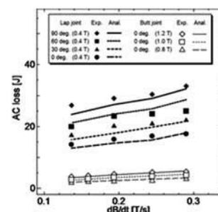
Fig. 2. AC loss of lap and butt joint
