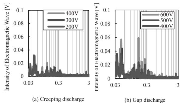
Fig.3. Frequency spectrum of radiation EM
