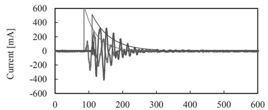
Fig.2. Example of measured PD current
