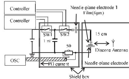
Fig. 1. PD generation and measurement circuit system
