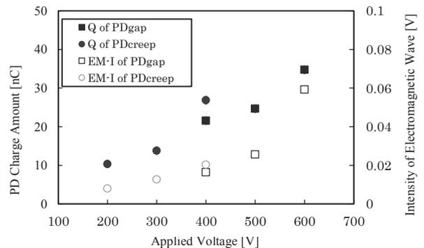
Fig. 4. The applied voltage dependence of EM intensity and PD charge amount by different discharge type
