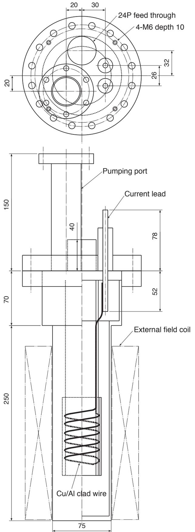
Fig. 1. Schematic drawing of a testing sample. A copper clad aluminum wire is wound on a plastic tube that is inserted in a vacuum chamber.
