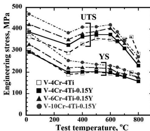
Fig. 1. Dependence of yield stress (YS) and ultimate tensile strength (UTS) on test temperatures.
