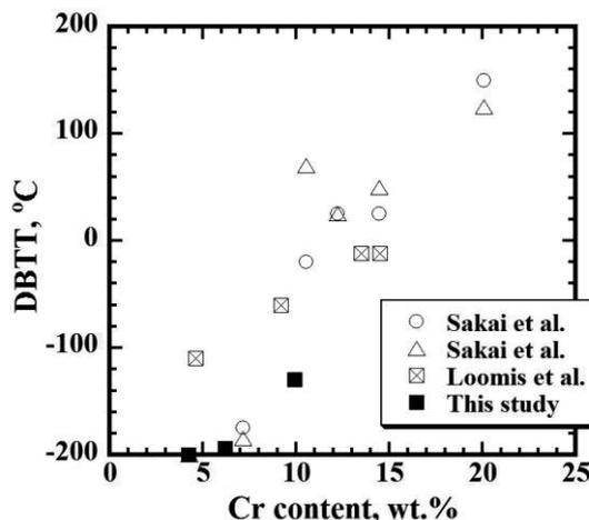
Fig. 3. Dependence of DBTT for V<sub>x</sub>Cr-(4-5)Ti and V<sub>x</sub>Cr-4Ti-0.15Y alloys on Cr content. Open circles and triangles represent V<sub>x</sub>Cr-4Ti alloys annealed to obtain a mean grain size of 17 μm, and at 950 °C, respectively [3]. Open squares with cross represent V<sub>x</sub>Cr-5Ti alloys annealed at 1125 °C [4]. Closed squares represent V<sub>x</sub>Cr-4Ti-0.15Y alloys annealed at 950 °C (this study).
