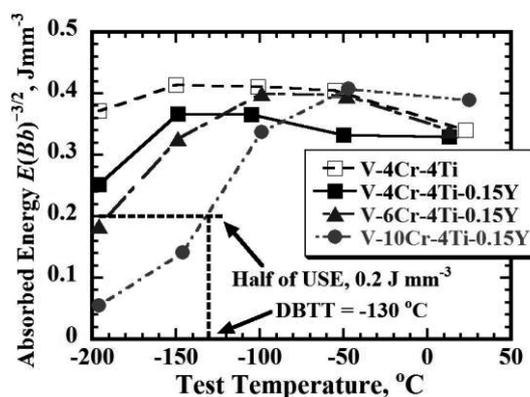
Fig. 2. Absorbed energies in the Charpy impact tests.
