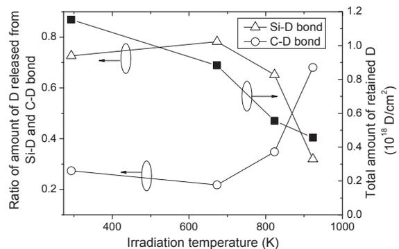
Figure 3 Total amount of desorbed deuterium, and the ratio of the amounts of desorbed  $D_2$  at the lower (Si-D bond) and the higher (C-D bond) temperature peaks.
