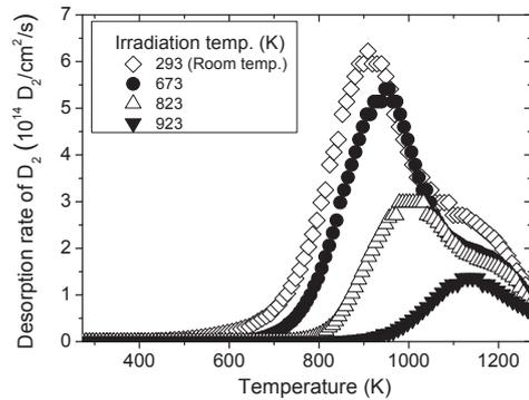
Figure 2 Thermal desorption spectra of  $D_2$  after deuterium ion irradiation at various irradiation temperatures.
