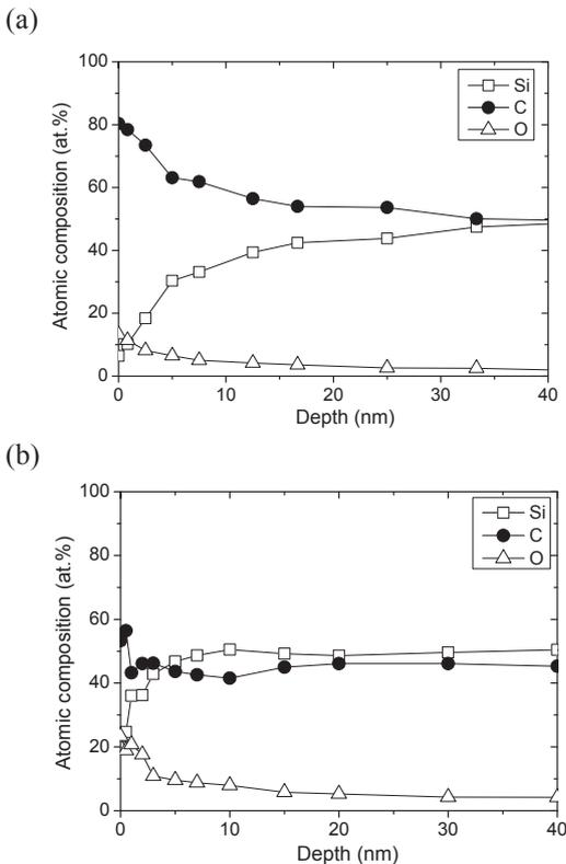
Figure 1 Depth profiles of the atomic composition of SiC/SiC composites before deuterium irradiation (a) and after deuterium irradiation at 673 K (b).
