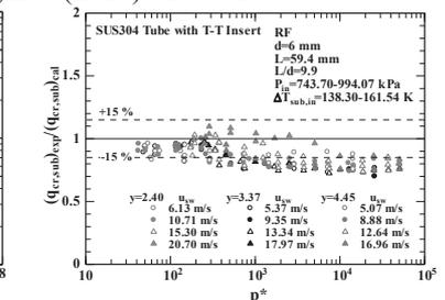
Fig. 4 Ratios of  $q_{cr,sub}$  for  $d=6$  mm with  $y=2.40$ , 3.37 and 4.45 (186 pts) to values calculated by Eq. (2) vs.  $p^*$
