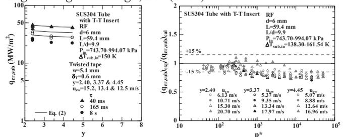
Fig. 3  $q_{cr,sub}$  vs.  $y$  for  $d=6$  mm with  $y=2.40$ , 3.37 and 4.45 on  $\tau=40$  ms, 165 ms and 8 s at  $\Delta T_{sub,in}=150$  K
