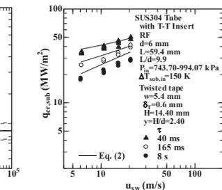
Fig. 2  $q_{cr,sub}$  vs.  $u_{sw}$  for  $d=6$  mm with  $y=2.40$  on  $\tau=40$  ms, 165 ms and 8 s at  $\Delta T_{sub,in}=150$  K
