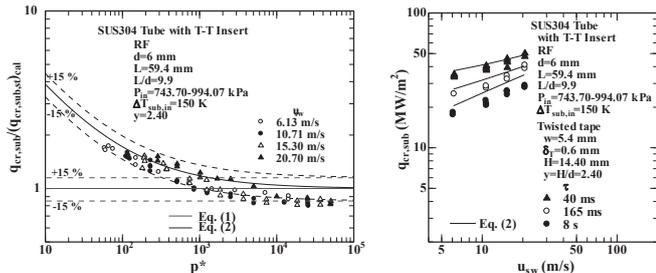
Fig. 1 Ratios of  $q_{cr,sub}$  for  $d=6$  mm with  $y=2.40$  (91 pts) to values calculated by Eq. (1) vs.  $p^*$
