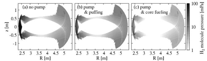
Fig. 1: Distribution of  $\text{H}_2$  molecule pressure of the closed divertor configuration.
