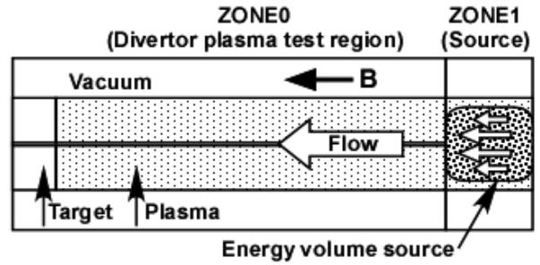
Fig. 1. Schematic of the NAGDIS-II plasma simulation.
