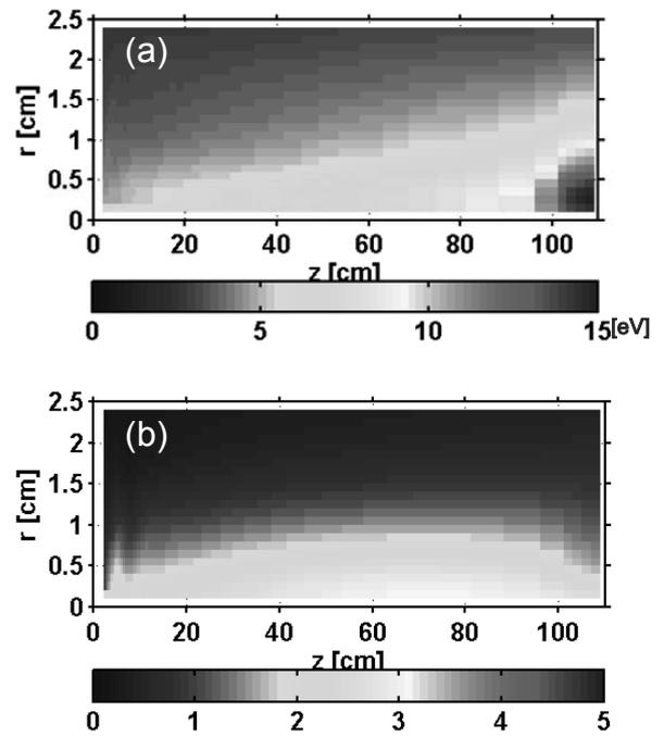
Fig. 2. Calculated distributions of (a) electron temperature and (b) electron density.
