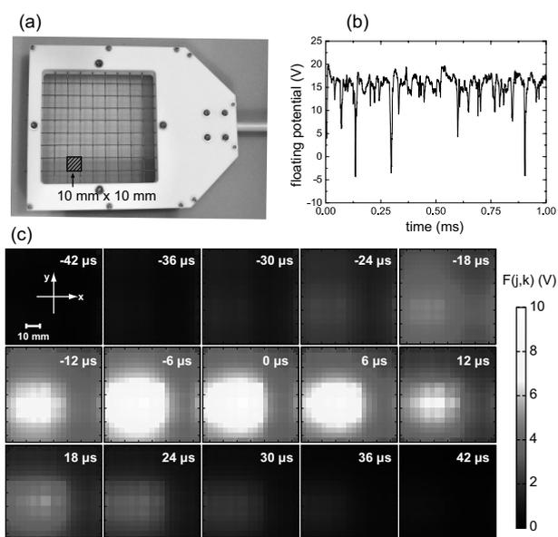
Fig. 1: (a): A picture of the HIWG detector, and (b): time series of floating potential. (c): Time slices of the reconstruction result.<sup>4)</sup>
