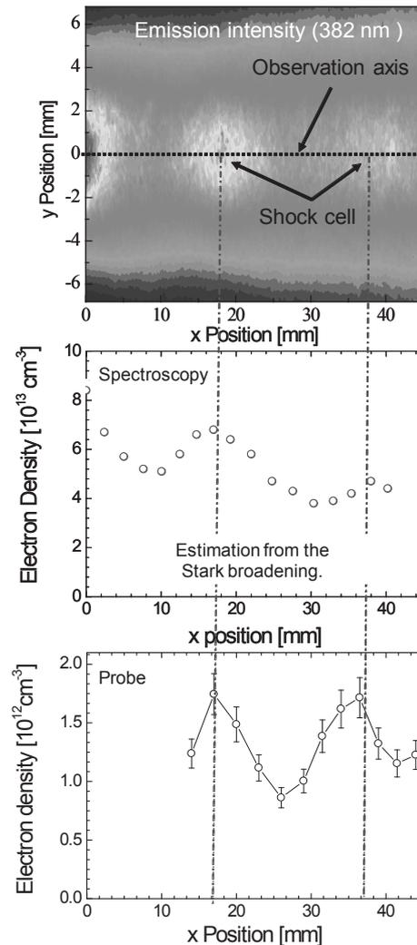
Fig. 1. Spatial variations of plasma parameters. From the top panel, the monochromatic emission image of He I 388 nm, electron densities determined by the Stark broadening spectra and probe measurements, respectively.
