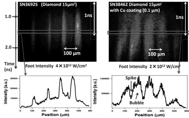
Fig. 1. Raw streaked image with face-on radiograph measurements with and without Cu coating.
