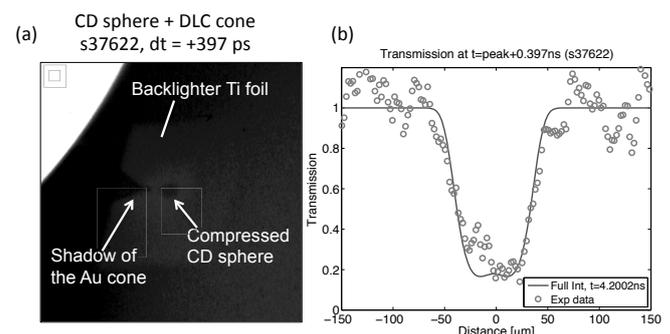
Fig. 2. (a) A monochromatic x-ray images of driven CD shell and (b) transmission profile of the driven sphere target.
