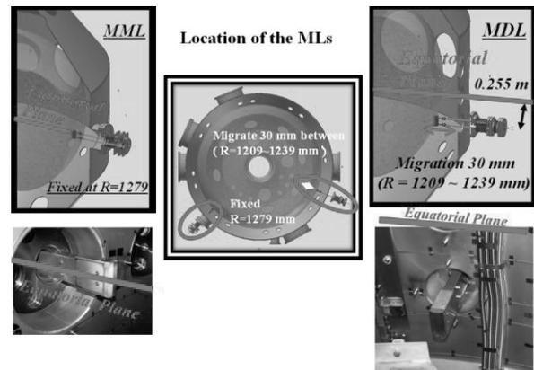
Fig. 1 Layout of the new movable limiter (MDL) and the existing movable limiter (MML). The center figure illustrates a top-cross-sectional view of the QUEST vessel and toroidal position of both MLs is clearly identified. Top-right and top-left show schematic pictures of MML and DML, respectively. Bottom-right and Bottom-left are the pictures of each ML.
