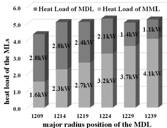
Fig. 2 Heat load distribution depending on the DML position is plotted, when the MML was located at  $R=1.279\text{m}$ . Top and bottom sides of each square prism correspond to the heat load to DML and MML, respectively. Every data was monitored with calorimetric technique for cooling water.
