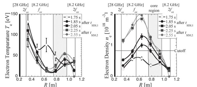
Fig. 3. Electron (a): temperature and (b): density profiles measured by Thomson scattering diagnostics in the 28 GHz and 8.2 GHz injections.
