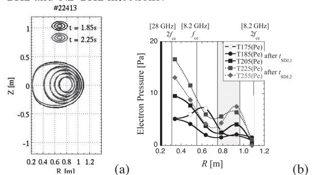
Fig. 4. (a): Magnetic flux surfaces analyzed by EFIT and (b) Electron bulk electron pressure profile in the 28 GHz and 8.2 GHz injections.
