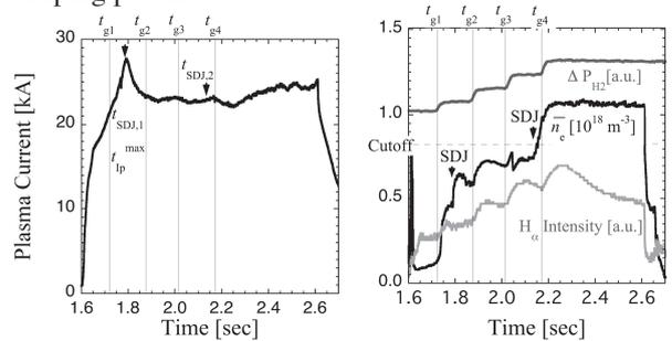
Fig.2. Time evolution of (a): plasma current and (b): hydrogen reservoir tank pressure, line-averaged density and  $H\alpha$  intensity in the 28 GHz and 8.2 GHz injections.
