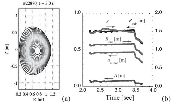
Fig.1. (a): Magnetic flux surfaces analyzed for the 54 kA plasma by EFIT. (b): Time evolution of the plasma shaping parameters.
