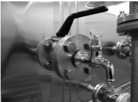
Fig. 22. Before drainage, water is sampled manually and measured with a low background liquid scintillation counter (LSC-LB7).
