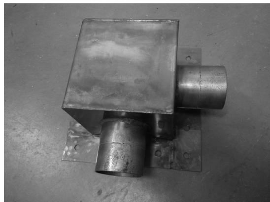
Fig. 2. Oxygen-free copper shield box.
