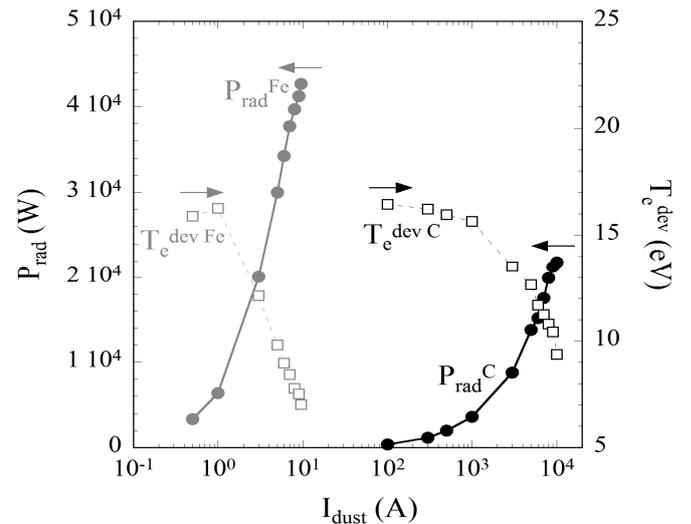
Fig. 2. Calculated radiation power and divertor electron temperature for iron and carbon dust emission as a function of the dust current.
