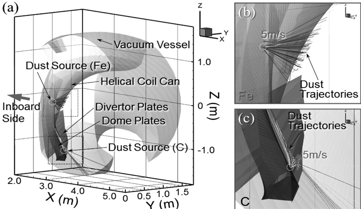
Fig. 1. (a) A perspective view of the LHD vacuum vessel and the closed divertor components for the simulation. The trajectories of iron dusts released from a helical coil can (b) and carbon dusts from a lower divertor region (c).
