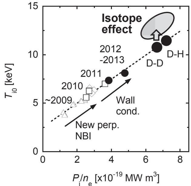
Figure 2. The comparison of  $T_{i0}$  between the previous achievement and the expected value in the deuterium experiments with regard to the ion heating power normalized by the electron density.
