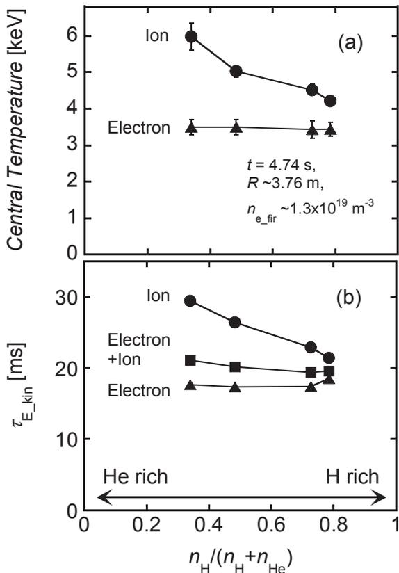
Figure 1. The dependence of (a) the central temperatures and (b) the energy confinement time for ion and for electron with four different conditions of H/He ratio.
