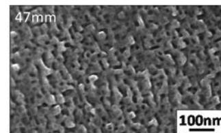
Fig. 2. FE-SEM images on the divertor strike point. Position is indicated on upper left side of the image, and it corresponds to the position on Fig. 1.
