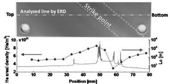
Fig. 1. Upper: photograph of the tungsten exposed to the ultra-long pulse He discharges. Lower: retention profile of He on the tungsten measured by ERD (diamond symbol), and typical connection length ( $L_c$ ) profile of magnetic field lines during He discharges.
