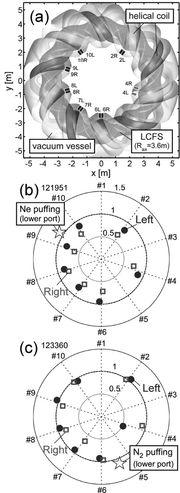
Fig. 1 (a) Top view of the toroidal divertor probe arrays. Polar plot of  $\Sigma I_{\text{sat}}$  ratios of before to after (b) Ne and (c)  $N_2$  puffs on L (filled circle) and R (empty square) plates. Toroidal positions of Ne and  $N_2$  puffing ports are also depicted (filled star).
