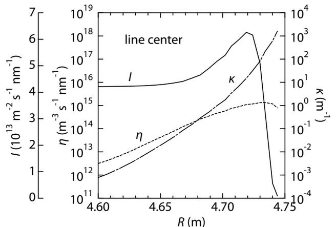
Fig. 2: Radial profiles of the emission coefficient  $\eta$  (dashed line) and absorption coefficient  $\kappa$  (dot-dashed line) at the line center evaluated from the Balmer- $\alpha$  line profile analysis. The resulting line intensity of the Lyman- $\alpha$  line at the line center is given by the solid line.
