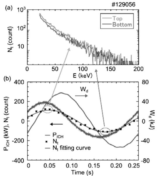
Fig. 1. Sinusoidal modulation experiment for investigating the heating characteristics of various antennae. By modulating the ICRF power, the modulation signals of high energy count  $N_t$  and plasma stored energy  $W_d$  were observed. (a) The effective temperature  $T_{eff}$  were almost the same at the top and the bottom of the sine curve.
