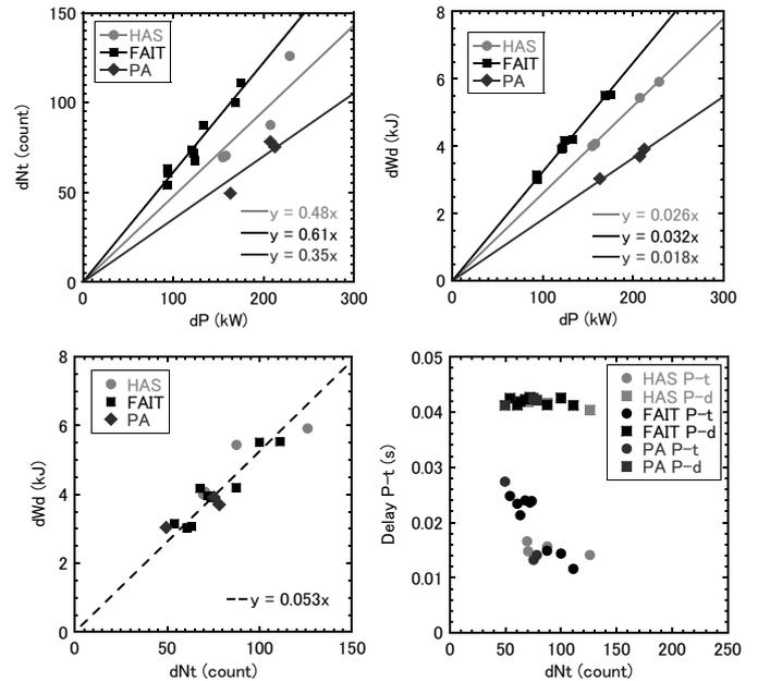
Fig. 2. Modulation amplitude of the  $N_t$  and  $W_d$  differed by the antenna type during the changing of the ICRF power  $P_{ICH}$ . On the other hand, the rate of generation of the tail and energy relaxation time were the same by the different antennae.
