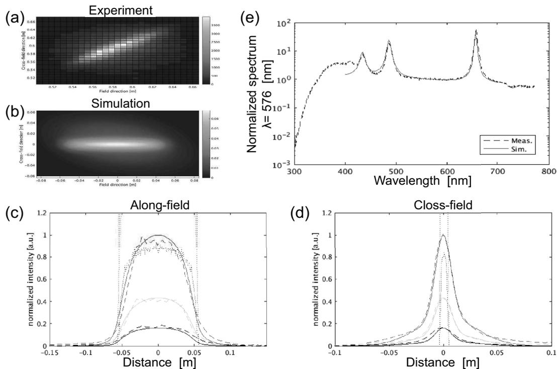
Fig. 1: Comparison between the experimental observation and computational analysis. (a) Fast camera image, (b) simulated light emission distribution, light emission profiles of  $H_\alpha$  (red),  $H_\beta$  (green) and  $H_\gamma$  (black) along-field (c) and cross-field (d) directions, and (e) visible spectrum. Measured and calculated values are denoted by dashed lines and solid lines, respectively.
