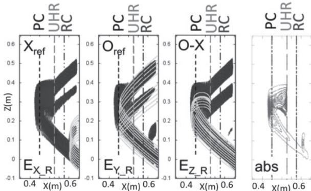
Fig. 1: Contours of the real components of the electric field ( $x, y, z$  from the left) and absorbed power obtained by full wave calculations when the injection angle set to be  $\theta_{opt}$ . Multi ray trajectories of the (from the left) reflected X-mode, the reflected O-mode, and the X-mode converted from the O-mode are drawn over.  $\theta_{inj} = \theta_{opt}$  at the beam center and  $\theta_{inj} = \theta_{opt} \pm 1.5$  at each edge of the beam.
