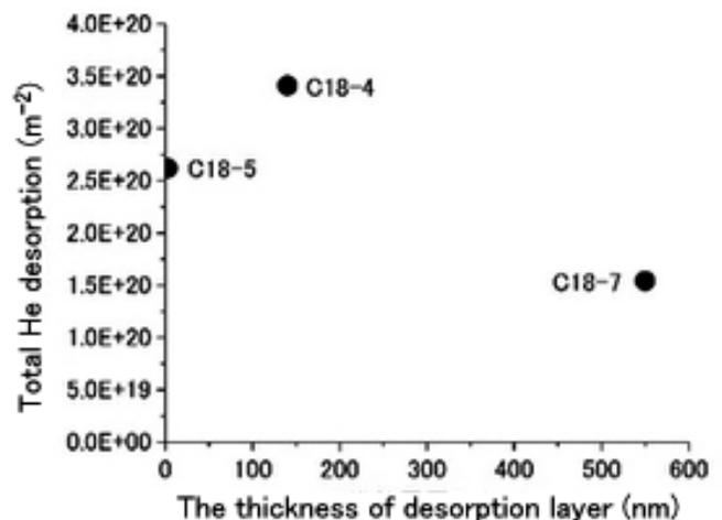
Fig. 2. The relation between the thickness of the mixed-material desorption layer from the cross-sectional TEM images and the total He desorption from SUS316L specimens.
