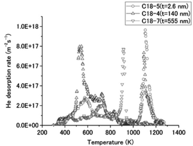
Fig. 1. Thermal desorption spectra of He obtained from the SUS316L specimens exposed to long-term plasma in LHD.
