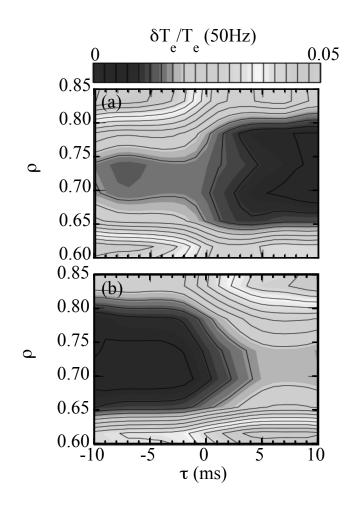
Fig. 1: Contour of relative modulation amplitude of electron temperature in space and time during the (a) forward transition (from high accessibility to low accessibility magnetic island) and (b) backward transition (from low accessibility to high accessibility magnetic island) at O-point.
