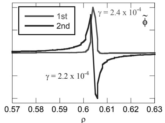
Fig. 3. Perturbation profiles of stream function  $\phi$  of first and second eigenfunction at  $p = 2$ .
