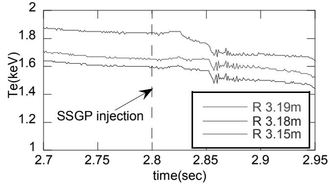
Fig. 1. Temporal evolution of electron temperature measured by ECE around SSGP injection time in #94655.
