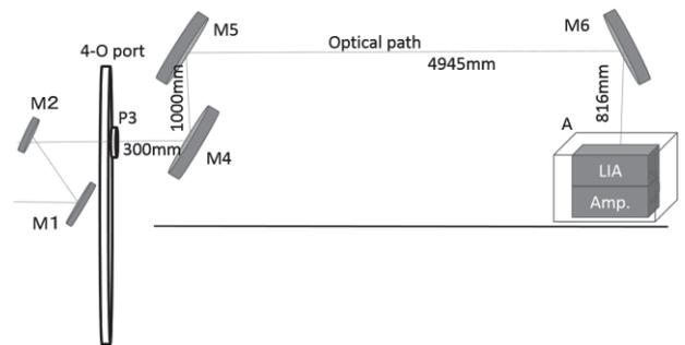
Fig. 2. Conceptual diagram of ECEI optical system (side view).
