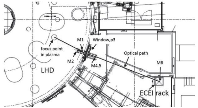
Fig. 1. Layout of ECEI optical system. This picture is a top view of LHD and measurement stage. Mirrors are indicated as M1, M2, M4, M5 and M6 on the optical path. P3 is the vacuum window.
