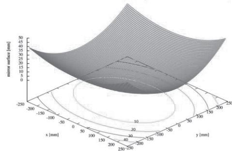
Fig.3. The M6 mirror surface designed by the concept of constant phase mirror.
