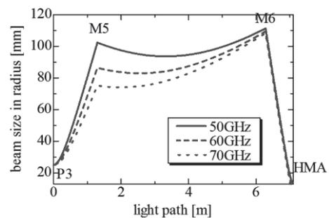
Fig.4 The development of designed beam radius from vacuum window (P3) to HMA.
