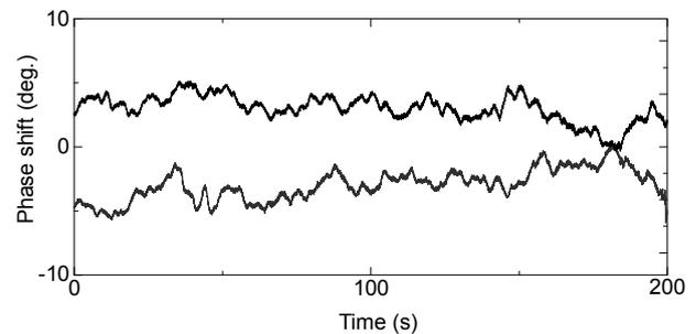
Fig. 3: Measuerd offset drifts of the low-power 1  $\mu\text{m}$  dispersion interferometer. Two data were acquired in different times.
