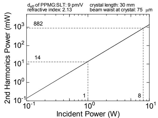
Fig. 2: Second harmonic generation with a high efficiency nonlinear crystal PPMgSLT.
