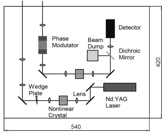
Fig. 1: Layout of a low-power 1  $\mu\text{m}$  dispersion interferometer
