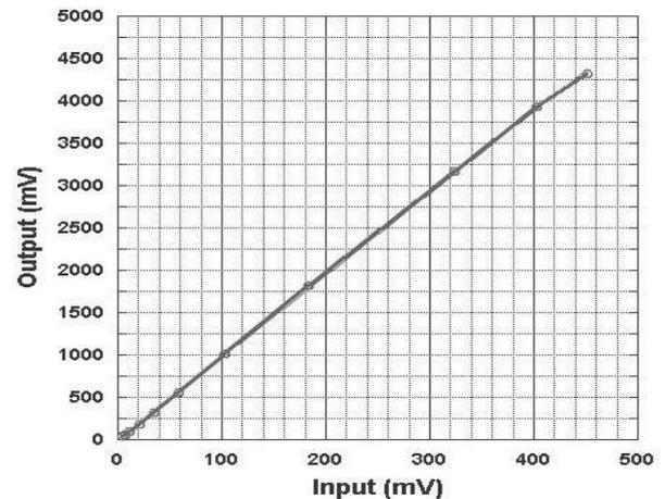
Fig. 3. Linearity of output response at the frequency of the input signal of 100 kHz.
