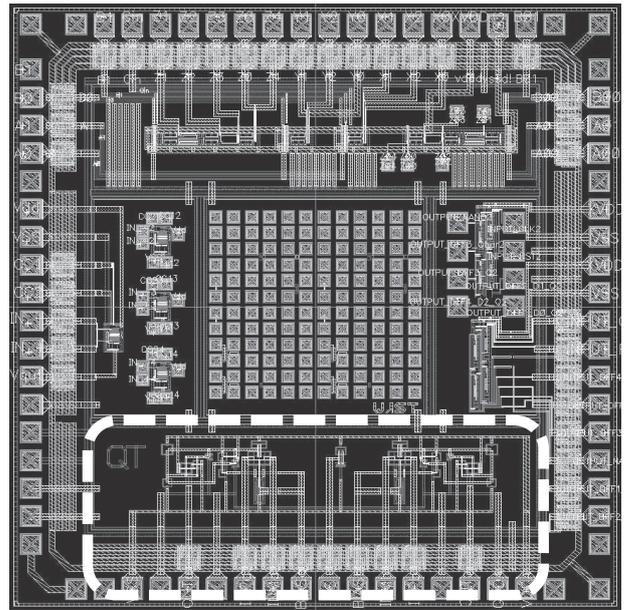
Fig. 1 A prototype of ASIC. The area enclosed by a white dashed curve consists of 2operational amplifiers.
