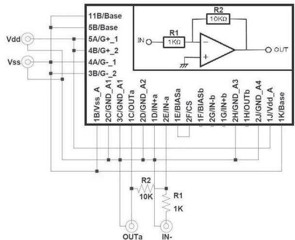
Fig. 2. Configuration of the test bench for evaluation test circuit of the prototype ASIC.
