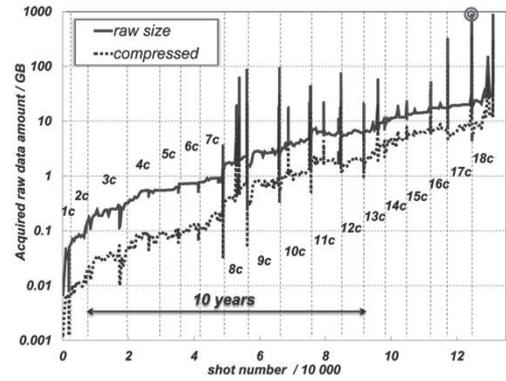
Fig. 1. Continuous data growth observed in LHD: Its exponential growth fits the Moore's law, *i.e.* 100 times in 10 years. Every Upper spike means the long pulse experiments, and the highest peak (double circled) corresponds to the world record of 891.6 GB/pulse.
