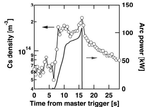
Fig. 3. Time evolutions of Cs density and arc power.
