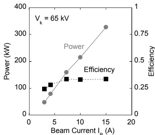
Fig. 1 Output power measured with a water load and efficiency as functions of the beam current. The beam voltage is 65 kV. Other parameters such as the modulation anode voltage are optimized for each beam current. The pulse width was set at 4  $\mu$ s.
