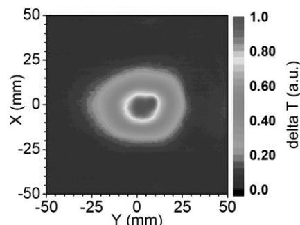
Fig. 2 Radiation pattern measured at a distance of 80 cm from the vacuum window flange. This pattern was obtained as temperature increase on a vinyl chloride plate measured with an infrared camera.
