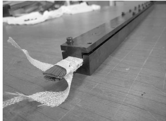
Fig. 2 Rutherford cable inserted in a stainless-steel case for the heat treatment.
