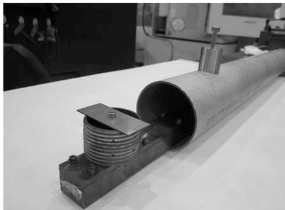
Fig. 3 Witness wire sample and Rutherford cable installing into the vacuum pipe for the heat treatment.
