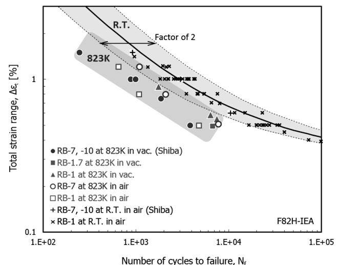
Fig. 1 Fatigue life of standard specimens (RB-7 and -10) and small specimen (RB-1) fabricated by F82H steel tested at room temperature and 823 K in air and in vacuum.
