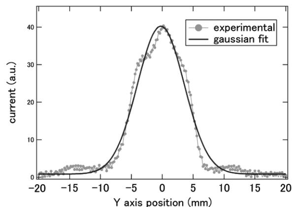
Fig. 1. Obtained beam profile by electrostatic probes.
