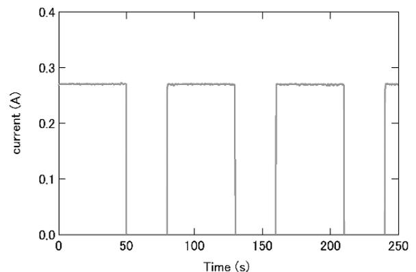
Fig. 2. An example of cyclic heat load test. The current is promotional to applied heat flux on the component.
