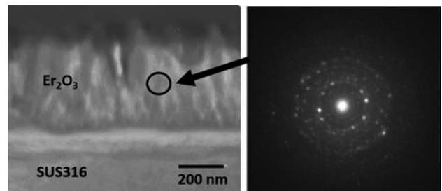
Fig.2 TEM image and SAED of the cross-sectional area on the  $\text{Er}_2\text{O}_3/\text{SUS}$  coating after  $\text{Cu}^{2+}$  ion irradiation at room temperature
