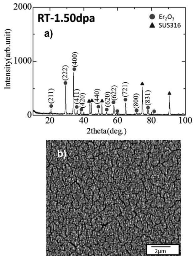
Fig.1 Typical XRD pattern and SEM image of the surface area on the  $\text{Er}_2\text{O}_3/\text{SUS}$  coating after  $\text{Cu}^{2+}$  ion irradiation at room temperature
