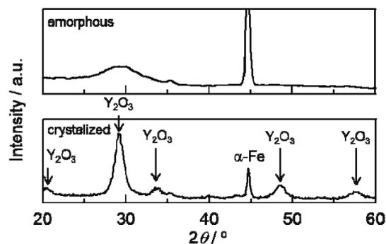
Fig. 2. XRD spectra of amorphous and crystallized  $Y_2O_3$  coatings.
