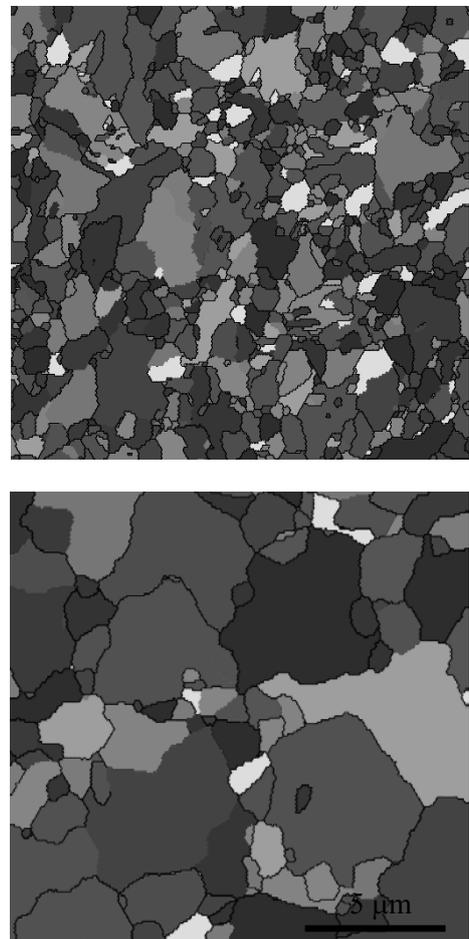
Fig.2 Microstructure by EBSD grain maps of 9Cr-ODS-1 (top) and 9Cr-ODS-2 (bottom) steels.
