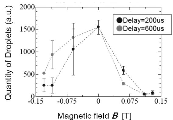
Fig. 2. Quantify of W droplets as a function of the external magnetic field strength in each direction.
