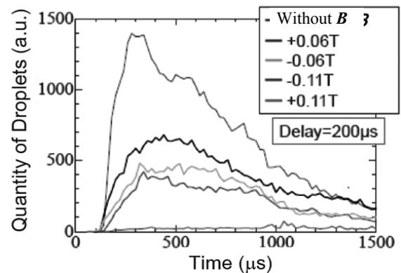
Fig. 1. Time evolution of quantify of W droplets in variation of the external magnetic field strength.
