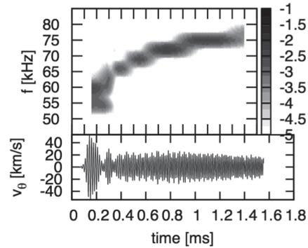
Fig. 1. The time evolution of EGAM oscillation (bottom panel) and frequency spectrum (top panel).
