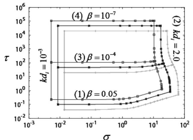
Fig. 1. Parameter space of the two-fluid effect and the beta value for tearing instability.
