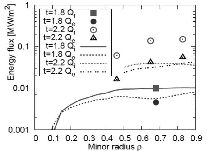
Fig. 3 Ion and electron energy fluxes due to turbulence,  $Q_i$  and  $Q_e$ . Symbols are from the simulations, and curves are from the experiments.
