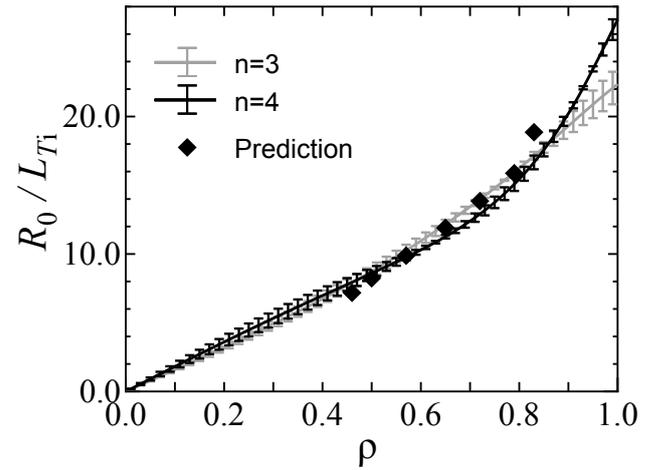
Fig. 1: Profiles of radial gradients of the ion temperature with the allowable ranges according to the experimental errors with the fitting functions  $T_i(\rho) = \sum_{k=0}^n c_k \psi^k(\rho)$  with  $n = 3$  (gray curve) and  $n = 4$  (black curve). The symbols represent the predictions of the temperature gradients by the flux-matching method.
