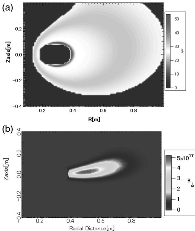
Fig. 1: Two dimensional spatial profiles of (a)  $T_e^{\text{cold}}$  estimated by 504.8/492.2 nm ratio and (b)  $n_e^{\text{cold}}$  estimated by 501.8/471.3 nm ratio.
