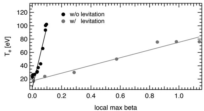
Fig. 2: Dependence of  $T_e^{\text{cold}}$  on local maximum  $\beta$  with and without levitation of the superconducting magnet.
