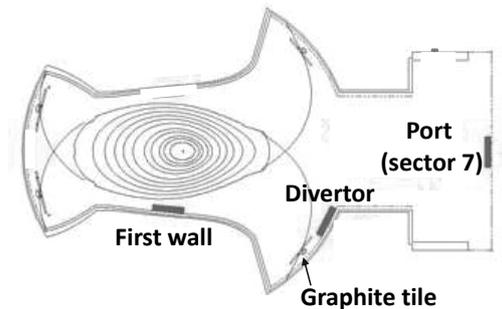
Figure 1 Poloidal cross section of the LHD and sample positions. ‘First wall’ sample was far from the graphite tiles and ‘Divertor’ sample close to the tiles. ‘Port’ sample was mounted only at toroidal sector 7.
