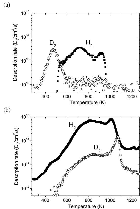
Figure 2 Thermal desorption spectra of H<sub>2</sub> and D<sub>2</sub> for the ‘First wall’ (a) and ‘Divertor’ (b) samples, which are located at toroidal sector 2 and 3, respectively.
