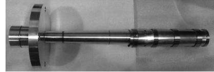
Fig. 1. Photo of Laval nozzle of SMBI installed in GAMMA10 central cell.
