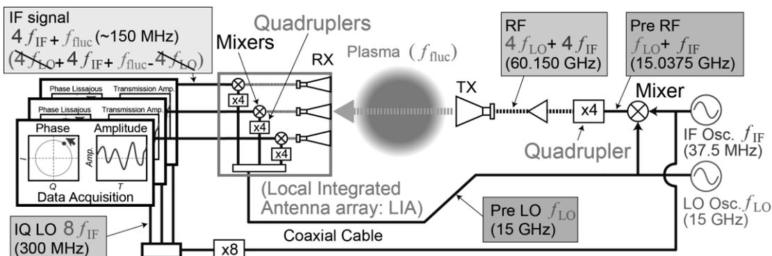
Fig. 1. Interferometer system using LIA.
