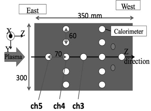
Fig. 1: Calorimeter channels of the lower V-shaped target. Distance of each channel is 7 cm.
