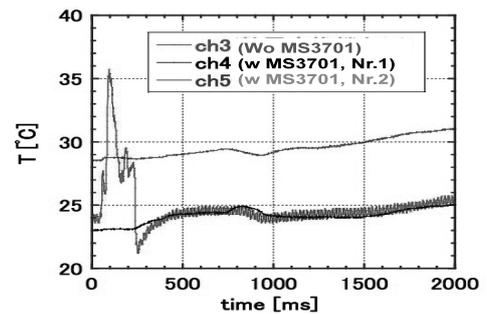
Fig. 3: Effect of Insulative converter MS3701 on thermocouple signal noise of V-shape target calorimeters.
