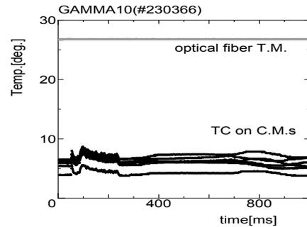
Fig. 2: Examples of thermocouple signal of V-shape target calorimeters. Test signal of optical fiber thermometer set near the west end of GAMMA 10/PDX.
