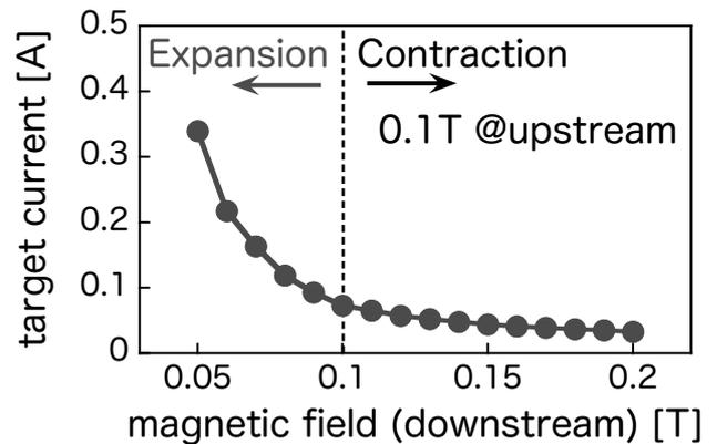
Fig. 2: Dependence of ion saturation current measured at the target plate on the magnetic field in downstream[1].
