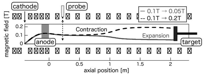
Fig. 1: Magnetic field strength at the center in a linear plasma device NAGDIS-II[1].
