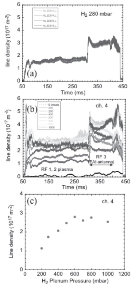
Fig. 2. (a) Line densities with H<sub>2</sub> gas plenum pressure at 280 mbar. (b) Time behavior of line density with different plenum pressure. (c) Plenum pressure dependence of line density.
