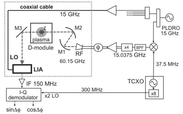
Fig. 1. New interferometer system with a local oscillator integrated antenna array (LIA).
